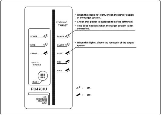
Figure 4.1 LED display when the power turned on
